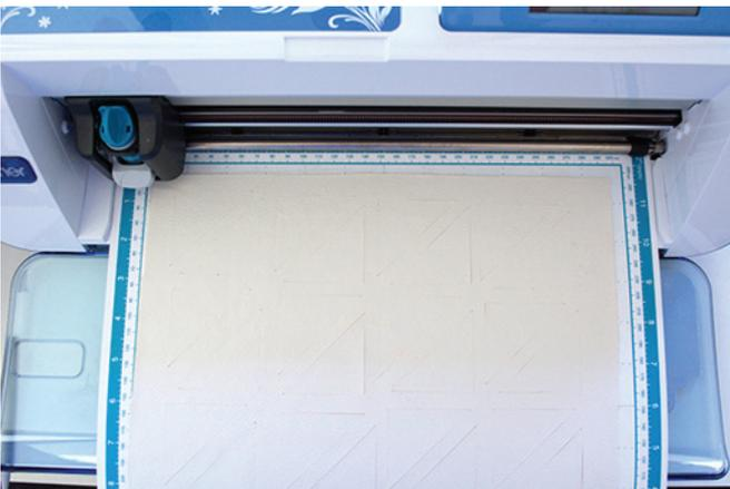
2. We used a high tac support sheet designed for sticking down fabric, which comes with the ScanNCut CM550DX machine and makes the process much easier. Place the high tac mat glossy side down onto the Standard mat, and then peel off the sticky layer. Place your vinyl down (leather look side up) and smooth out any wrinkles.
