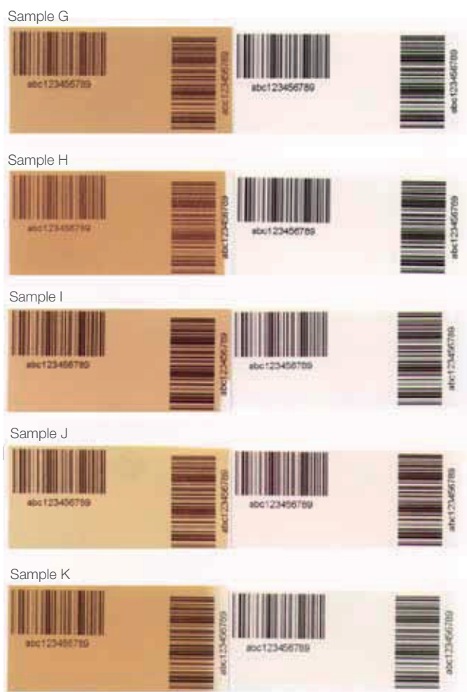
Figure 5 U.V light exposure seven-day test results
