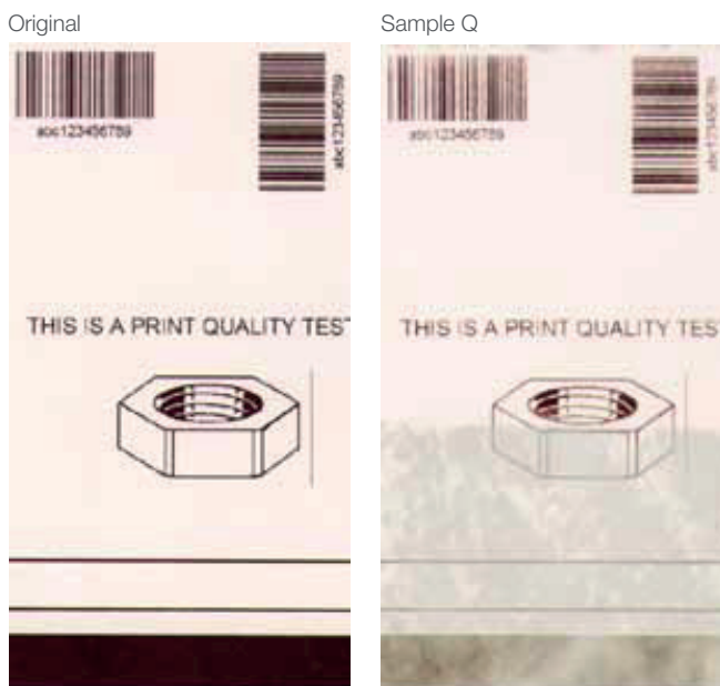
Figure 7. Plasticiser test results for shrink wrap
