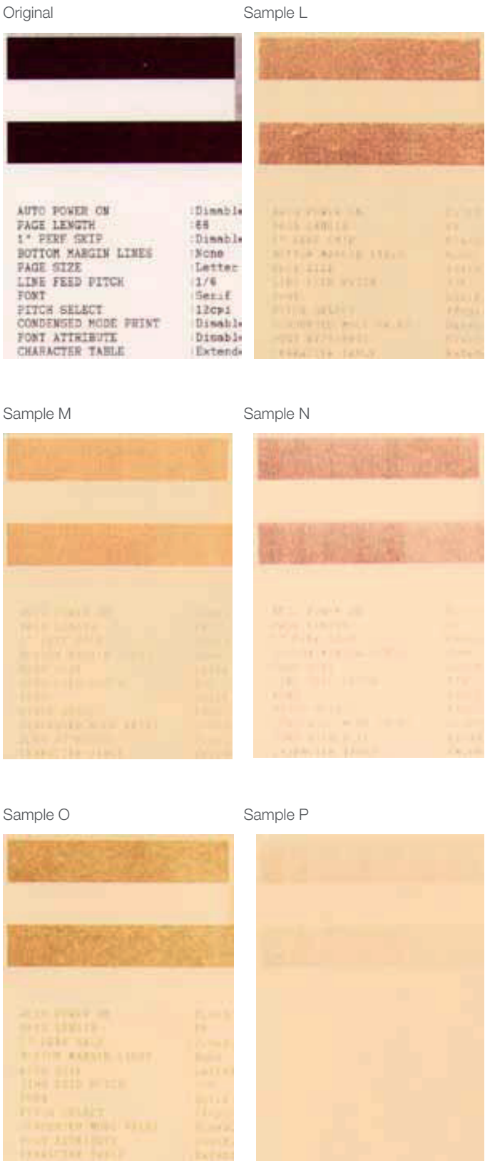
Figure 6 Long-term dashboard test results
