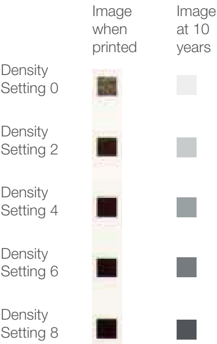
Figure 2. Printer density settings and image life
