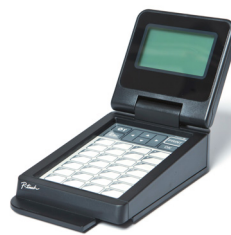
PA-TDU-003 Touch Panel display unit for stand-alone printing of labels (PT-P950NW only)
