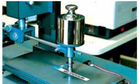
Abrasion resistant: after a 1kg sanding device was passed over the laminated labels 50 times, the text was unaffected
