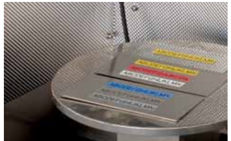
Fade resistant: after laminated labels were placed in a fade-inducing chamber to simulate a year in sunny surroundings, the text was unaffected
