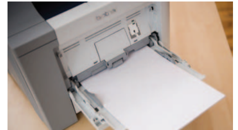
Multi Purpose Tray Print envelopes and labels using the multi purpose tray
